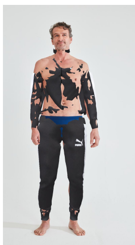
Figure 14. Bad case of Z-fighting, caused by the triangles of the occluder mesh sharing positions with the garment mesh.
