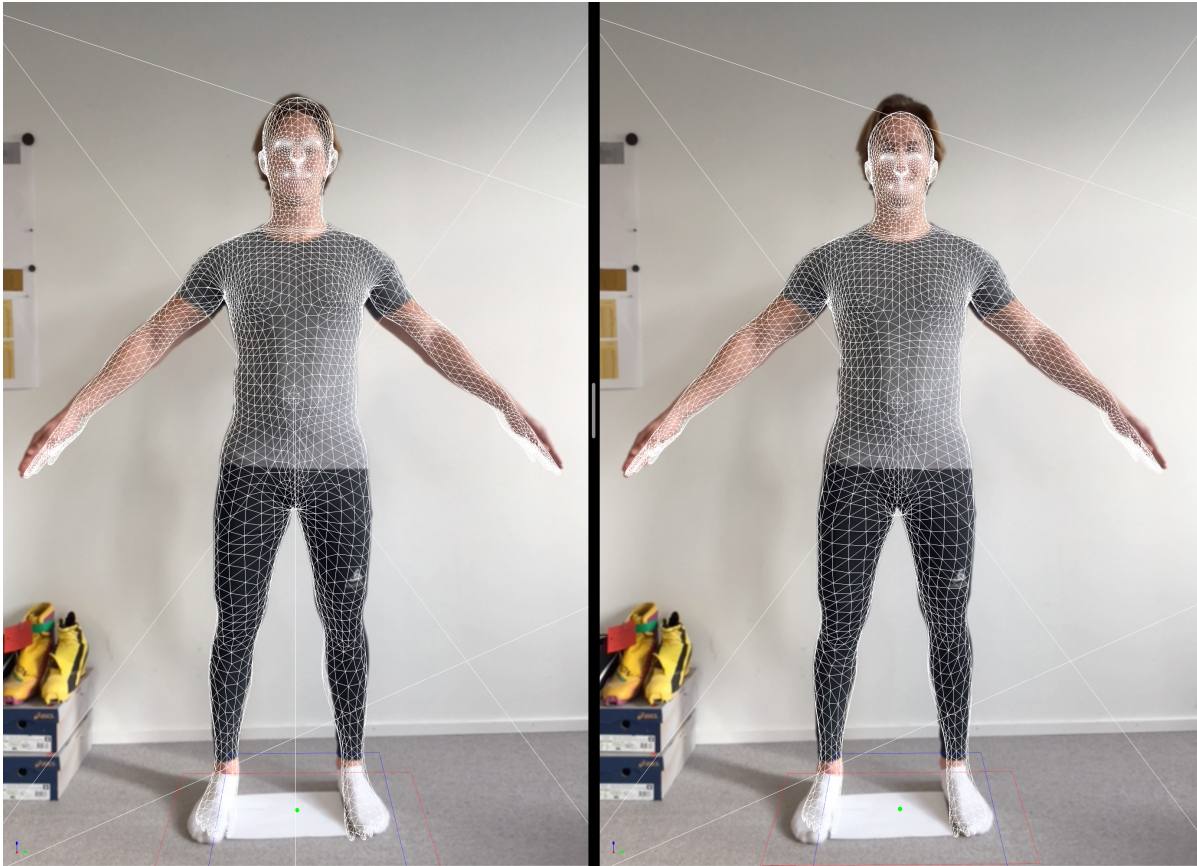
Figure 2.12: Matched avatar for model A.. Left: current method, Right: Improvement by segmenting head and hair.
