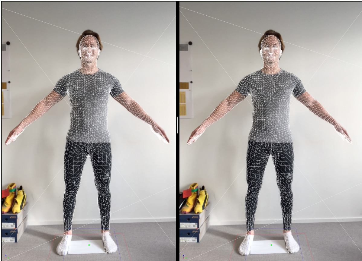
Figure 2.14: Matched morphed avatar for model A . with hair/head segmented. Left: 10 shape parameters. Right: 100 shape parameters. The fit to the image is better with 100 parameters, but we found experimentally that the accuracy in measurements is lower.
