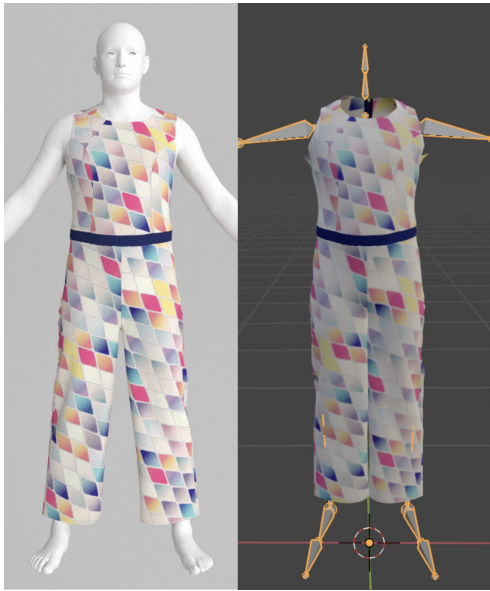
Figure 7: Garment simulated on avatar in VStitcher (left) and result after skinning and re-posing (right).
